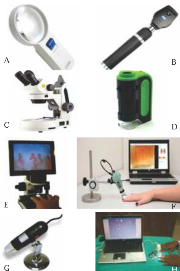
Fig 1. Instruments for NFC A- Magnifying glass; B- Ophthalmoscope; C- Stereomicroscope; D- Hand held microscope; E- Nailfold video capillaroscope; F- Capillaroscope; G & H- USB digital microscope
